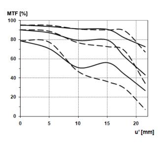
Modulation transfer MTF as a function of the image height (u') and slit orientation. White light. Spatial frequencies R=10, 20 and 40 cycles/mm.
